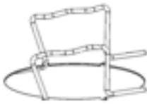
Slide the closed end of the Spring Clip into the bracket central opening.
