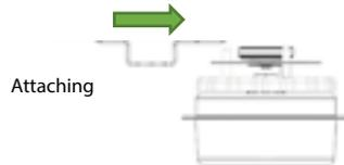
Align the bracket with the EcoBurner and push firmly, level and parallel to the base, forcing the spring arms apart.
