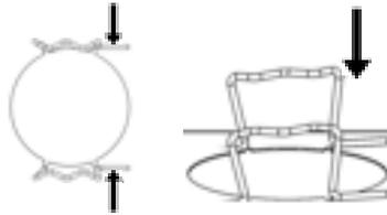
Squeeze the protruding open ends of the Spring Clip together and push these down into the central opening.
