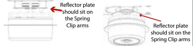
The EcoBurner reflector plate should sit on the Spring Clip arms and be held firmly in position.
