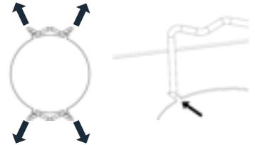
Ensure all four legs of the Spring Clip are held within the slots as shown.
